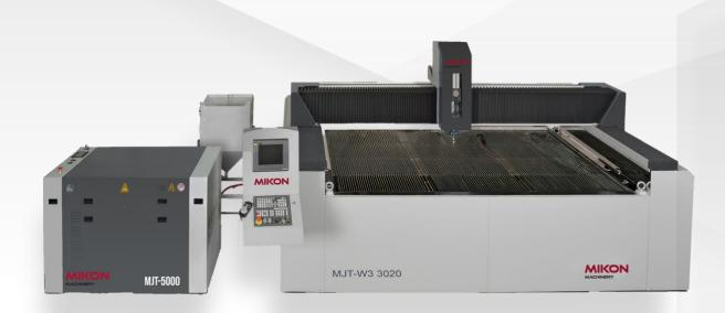
3 Axis CNC Waterjet can cut all kinds of materials existing in nature up to 200 mm thickness with power generated by mixing pressurized water and abrasive sand. All cutting materials can be made with the same nozzle. Not only for thick but also for thin materials, it can realize 90 degrees corners, narrow angular and small radius precise cuttings.
